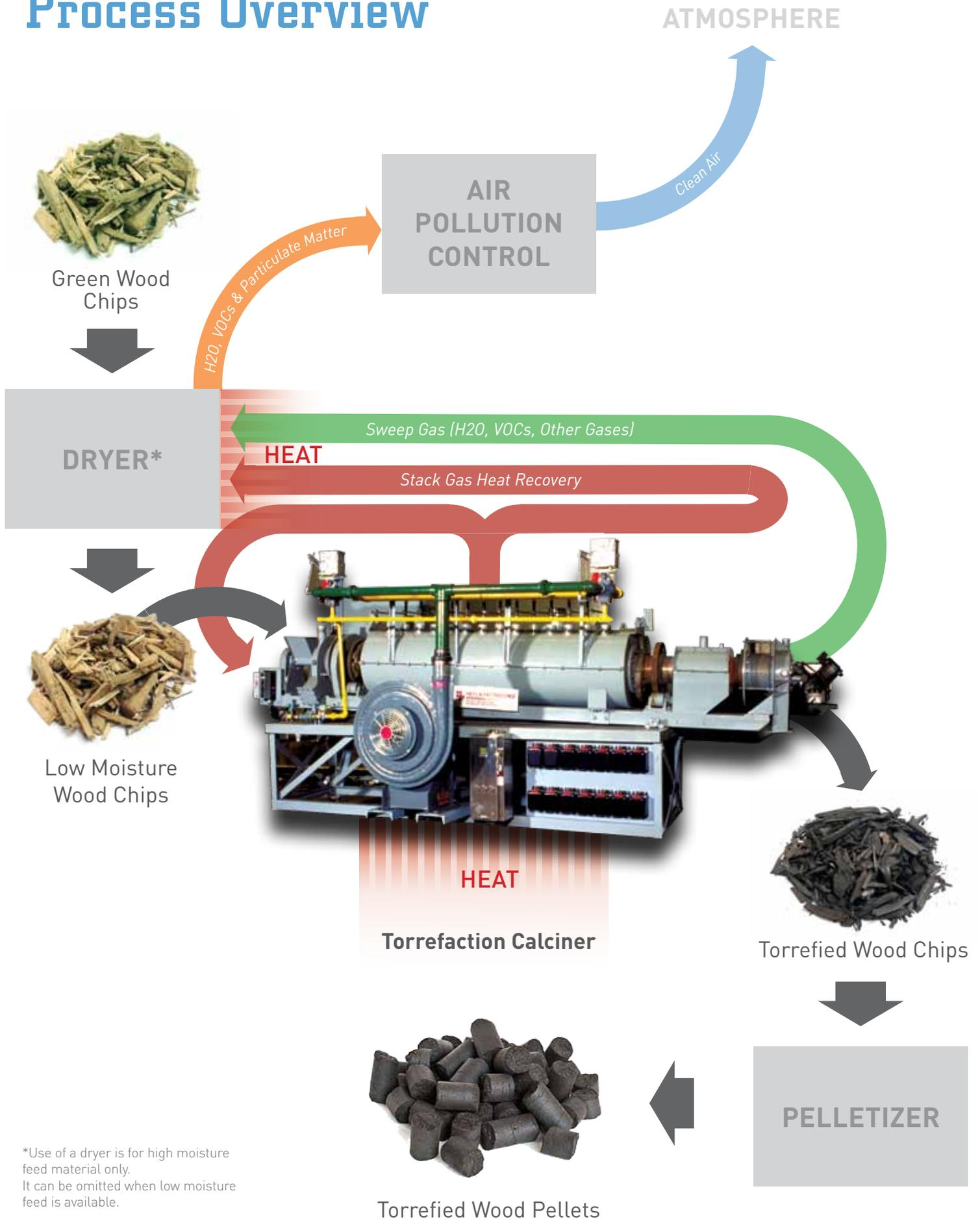
\*Use of a dryer is for high moisture feed material only. It can be omitted when low moisture feed is available.
