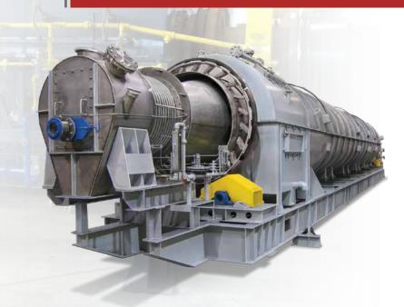
Co-current and counter-current material/ gas flow designs with multiple heating zone configurations are available. Integrated coolers provide cooling of product prior to discharge.
