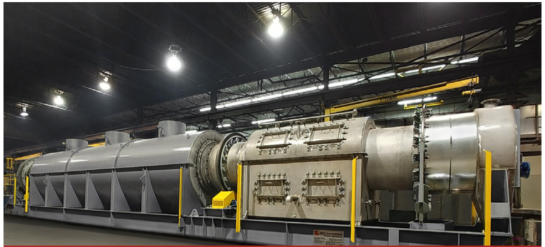
Heyl Patterson Rotary Calciners are available in designs from 4 inches to over 10 feet in diameter and lengths in excess of 100 feet.
