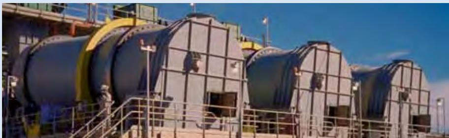
Rotary Agglomerator/Granulators Used to Process Copper
