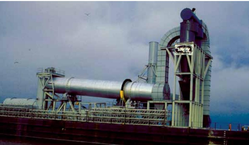
Barge-Mounted, Mobile Rotary Dryer Used to Process Bauxite
