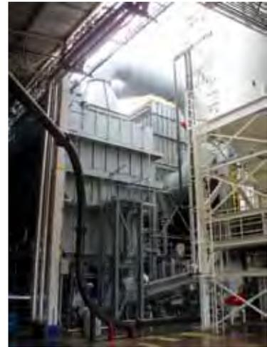
Fluid Bed Dryer Used for Spent Grain
