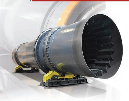
Alternating 45° and 90° tip flights in all rows provide uniform showering over the shell cross-section. Alternating rows of flights provide uniform showering along the shell length. This prevents short circuiting of the gas through the shell to minimize reductions in drying performance.
